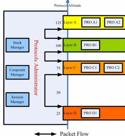
Figure 1 Packet Flow Chart of ABA
