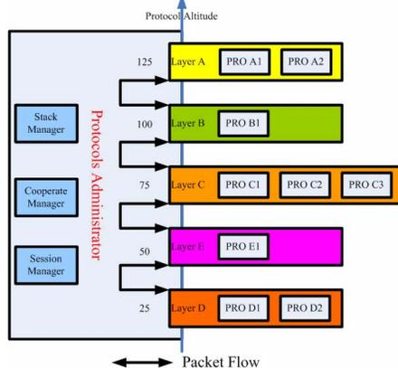
Figure 2 Packet Flow Chart of ABA with a new layer
