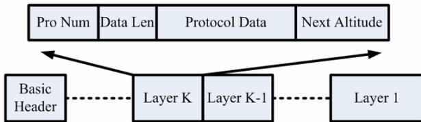
Figure 5 ABA Packet format
