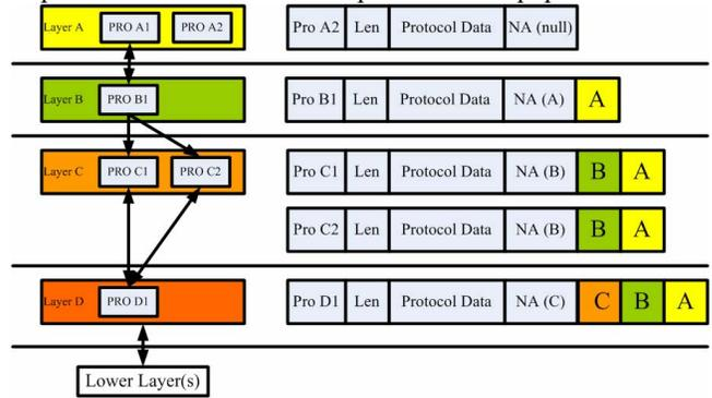
Figure 6 ABA processing sequence
