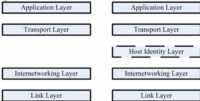
Figure 8 New Host Identity protocol layer
