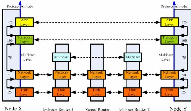
Figure 9 routing illustration of multicast packet
