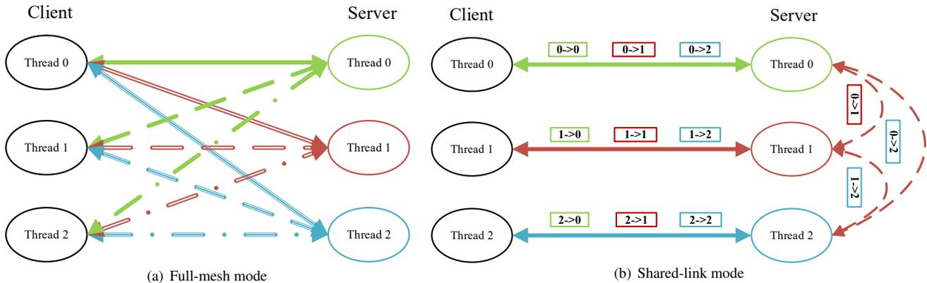
Figure 6: Different link modes for send/receive RPC requests
