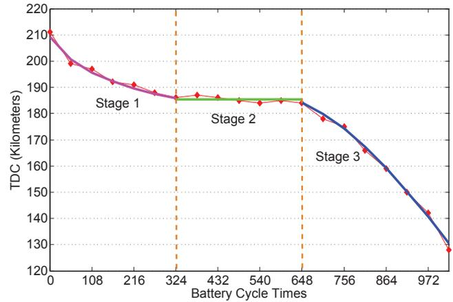
Fig. 7. Battery Degradation Curve In Real-life EV Use
